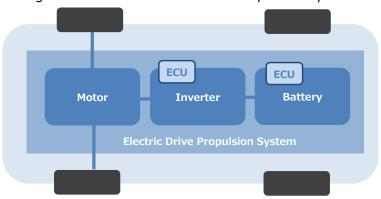
Figure: Outline of Electric Drive Propulsion System
